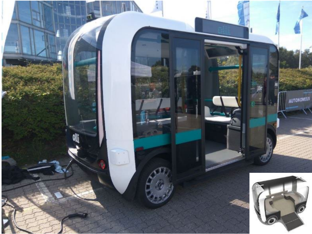
Olli by LM Industries, Local Motors, 3D printed car 速度25km/h (olli 最大40km/h)
