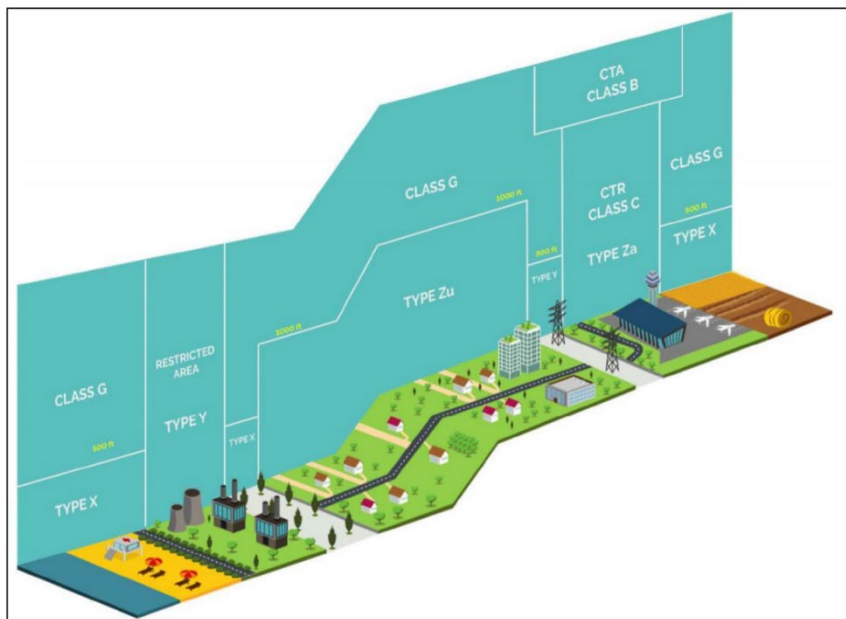
Fig. 12. SESAR's U-space airspace concept [145]. X – low risk, Y – medium risk, Z – highest risk.
