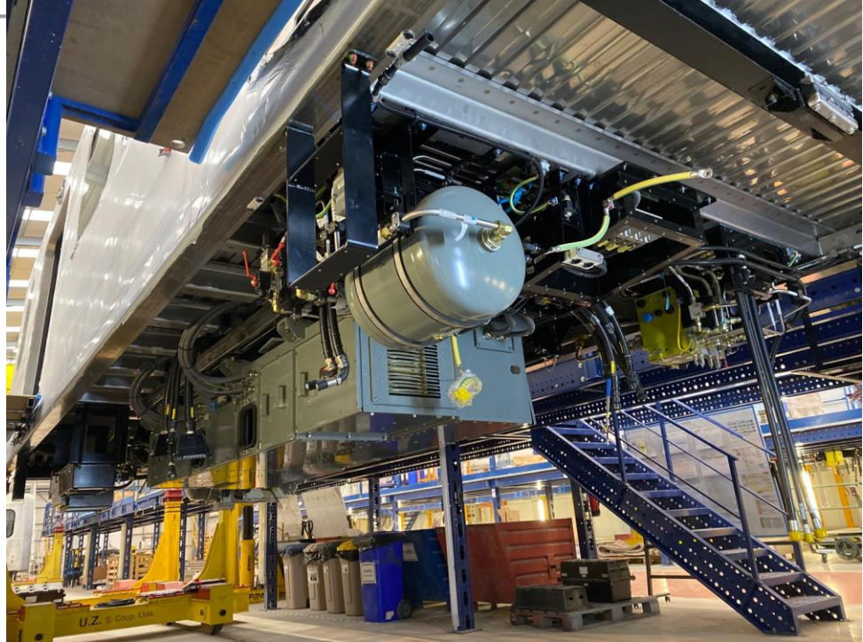
Underframe Equipment Assembly in CAF Trenasa Factory
