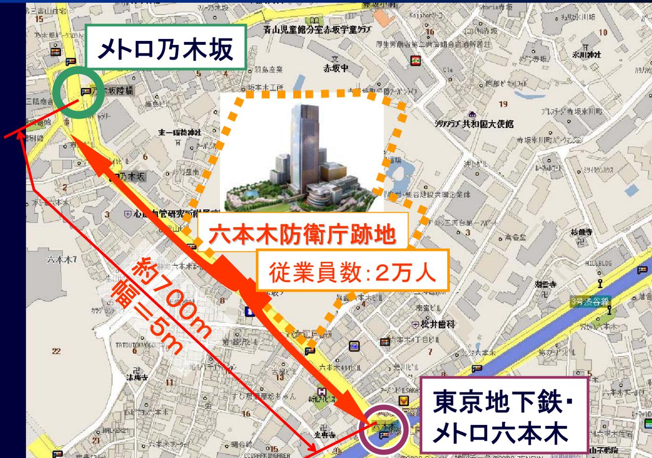
$$\frac{20,000(\text{人})}{700(\text{m}) \times 5(\text{m})} = 5.7 (\text{人}/\text{m}^2) \cong 200\% (\text{車内混雑率})$$
