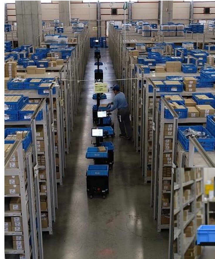
Supports picking operations while operating safely alongside human workers
