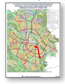
$\checkmark$  The length is 8.5 km (5km underground, 3.5km at-grade), there are 7 stations
