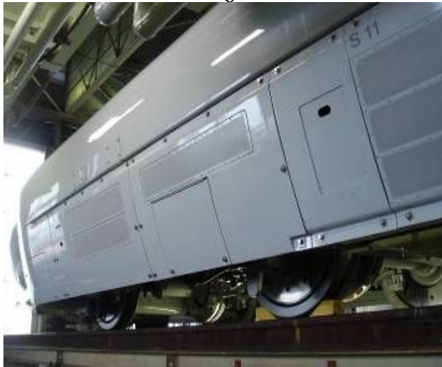
Full bogie cover & sound-absorbing panels
