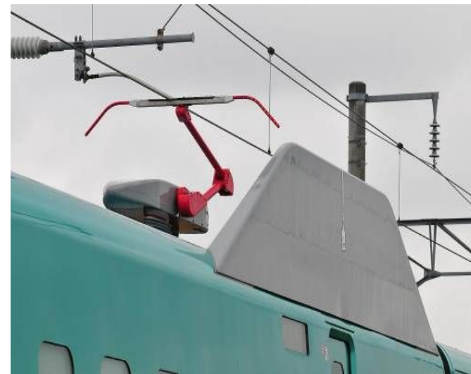
Pantograph noise insulation panels
